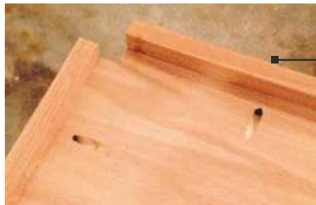
STEP 4. Reinforce the finished edges to the top with pocket holes, using the Kreg jig
